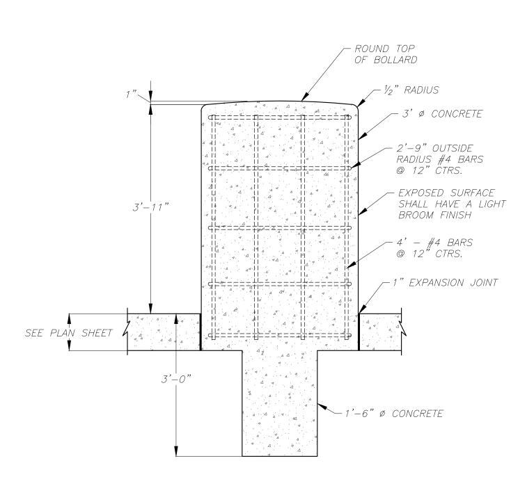
CONCRETE BOLLARD DETAIL
