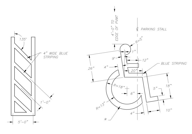
PAVEMENT MARKING SHALL BE A FAST DRYING, WATER BASED, ACRYLIC RESIN TYPE PAINT CAPABLE OF WITHSTANDING AIR AND ROADWAY TEMPERATURES WITHOUT BLEEDING, STAINING, DISCOLORING, OR DEFORMING AS MANUFACTURED BY SHERWIN WILLIAMS OR EQUAL.
